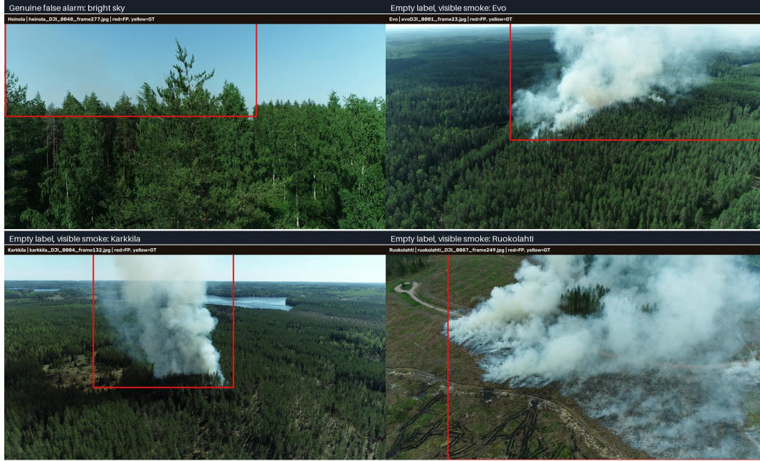
Figure 5: Selected error examples at 320 \times 180 . Predictions are shown in red and ground-truth boxes, when present, in yellow. The Heinola example is a genuine false alarm, while the other examples contain visible smoke that was not annotated.
