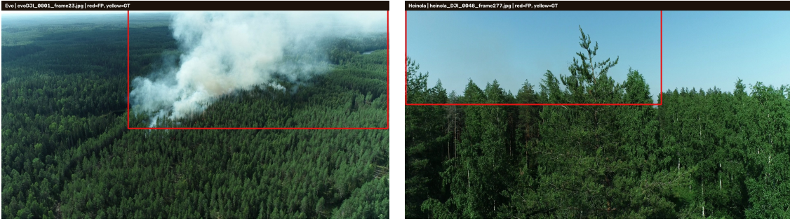
Figure 4: Examples from the error analysis. Left: visible smoke was detected but was missing from the ground-truth annotation. Right: bright, hazy sky was incorrectly detected as smoke.
