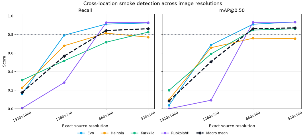
Figure 3: Recall and mAP@0.50 across the four tested image resolutions. The dashed line shows the macro average and the dotted line marks the 0.80 performance threshold.
